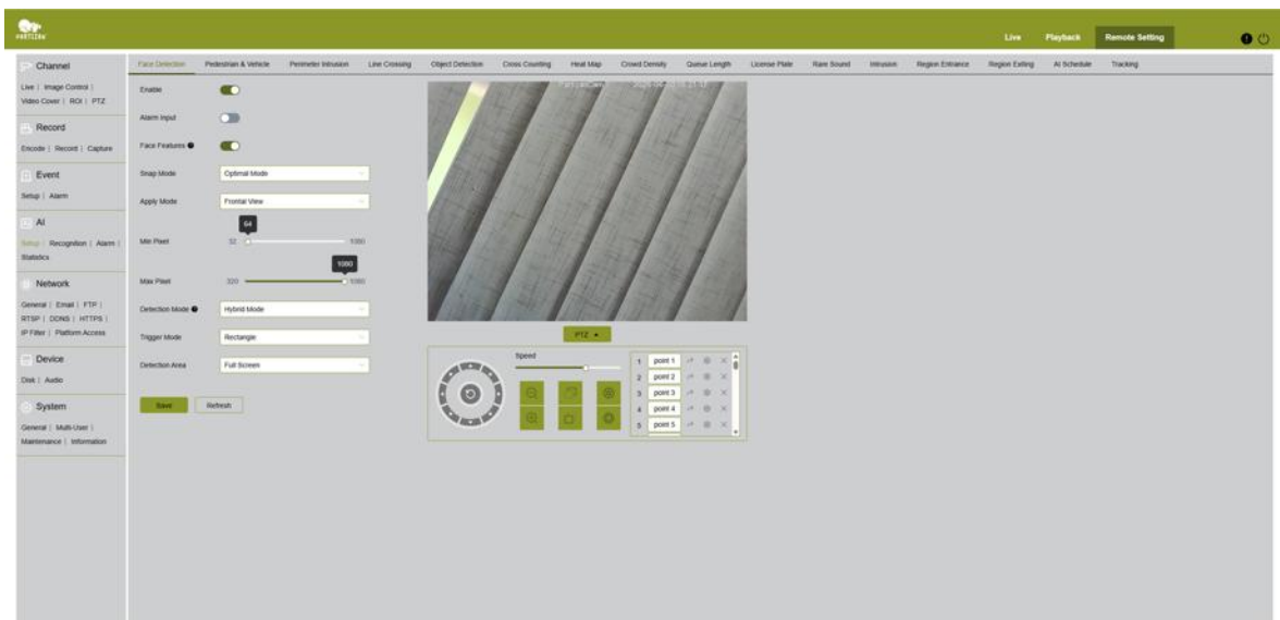
Fig. 38. AI → Setup → Face Detection — snap mode, apply mode, pixel range, detection mode, and trigger mode
