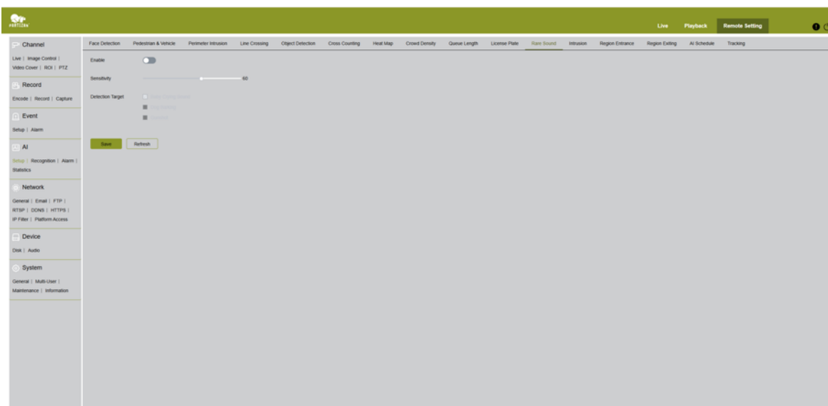
Fig. 48. AI → Setup → Rare Sound — sensitivity and detection target (Crying, Dog Barking, Gunshot)
