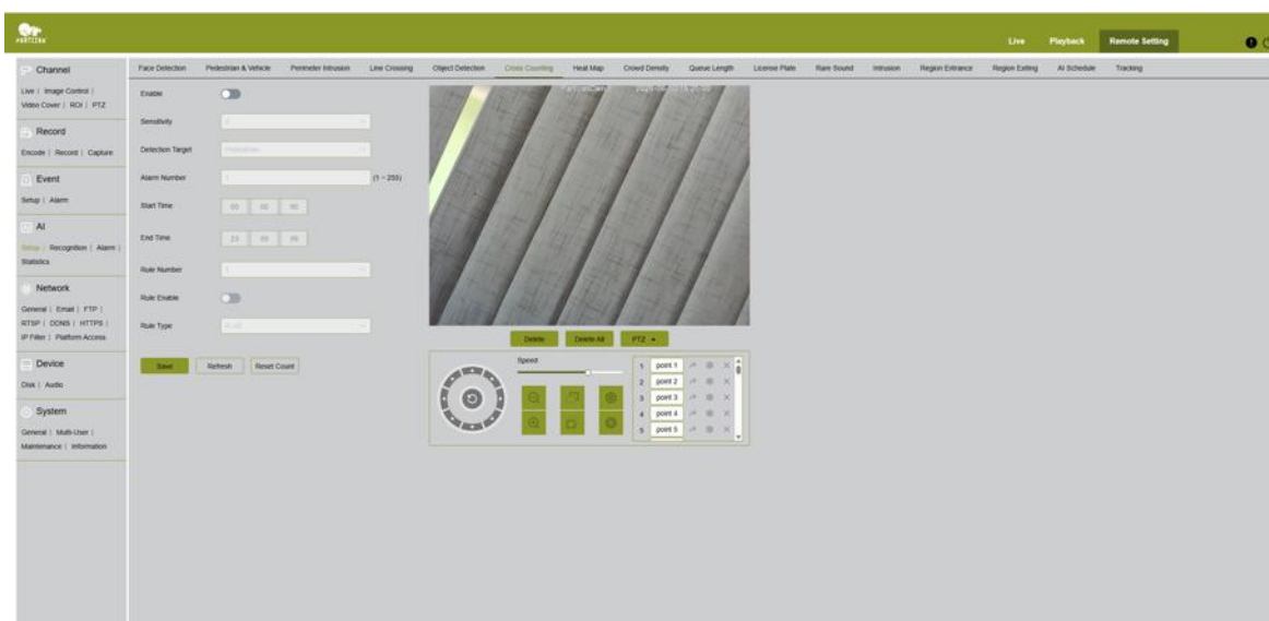
Fig. 43. AI → Setup → Cross Counting — counts crossings by target type, with start/end time and reset option
