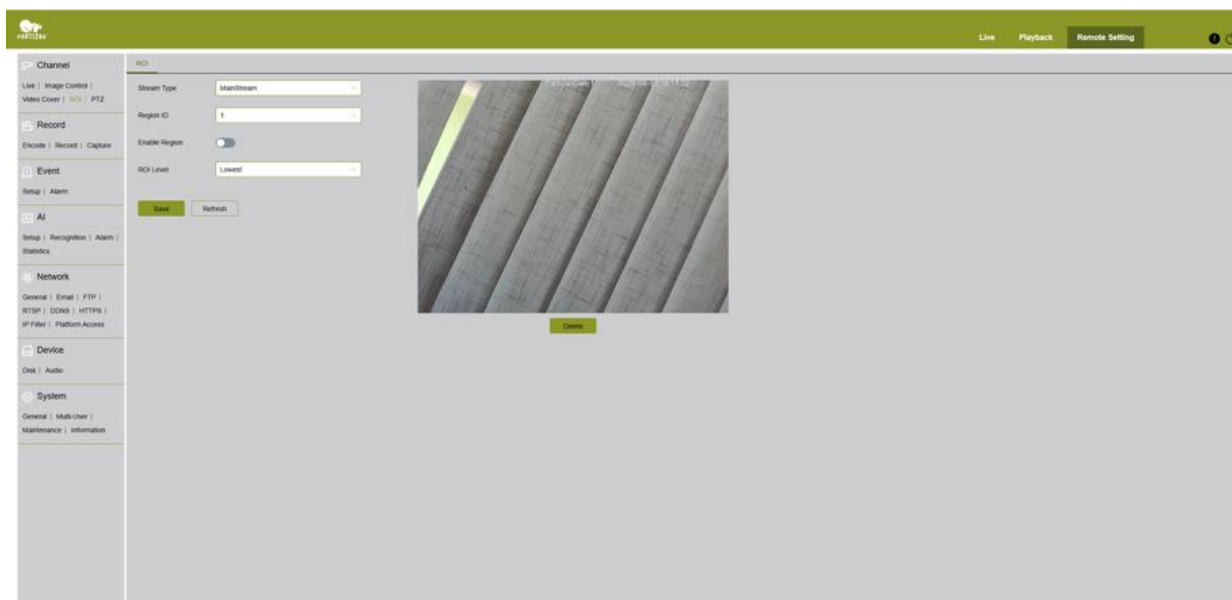
Fig. 21. Channel → ROI — stream type, region selection, and ROI quality level
