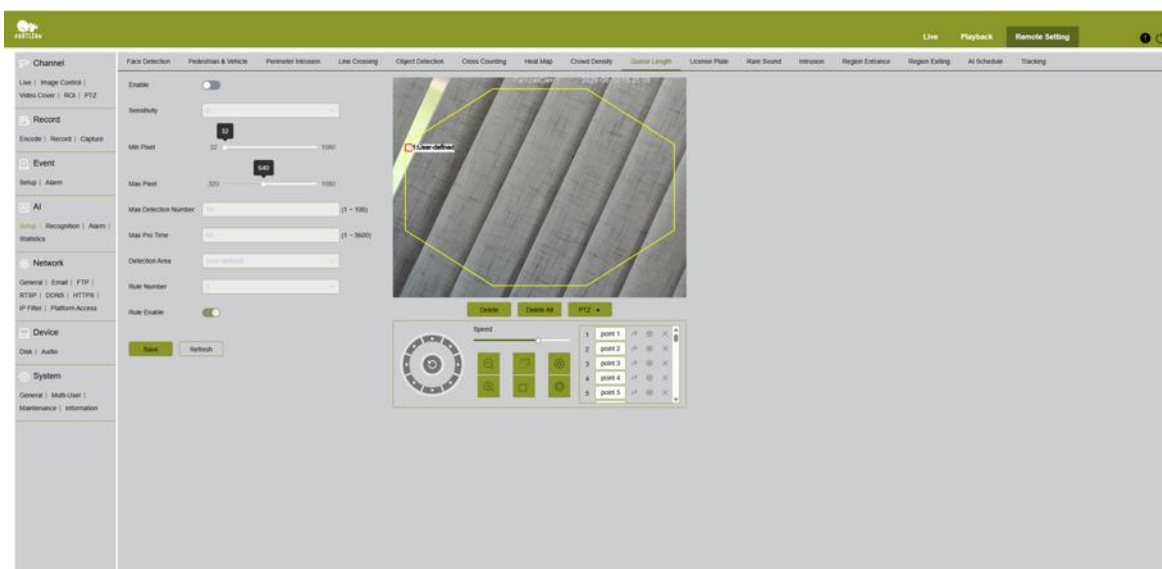
Fig. 46. AI → Setup → Queue Length — max detection number and maximum processing time
