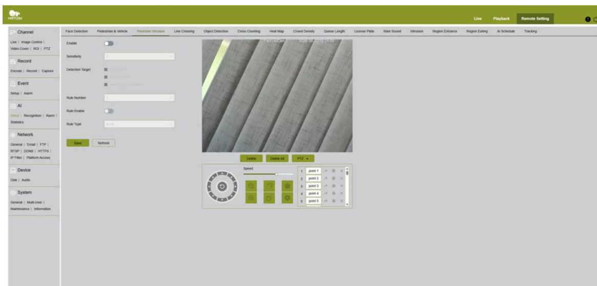
Fig. 40. AI → Setup → Perimeter Intrusion — draw a perimeter line on the preview and set rule direction (A→B)
