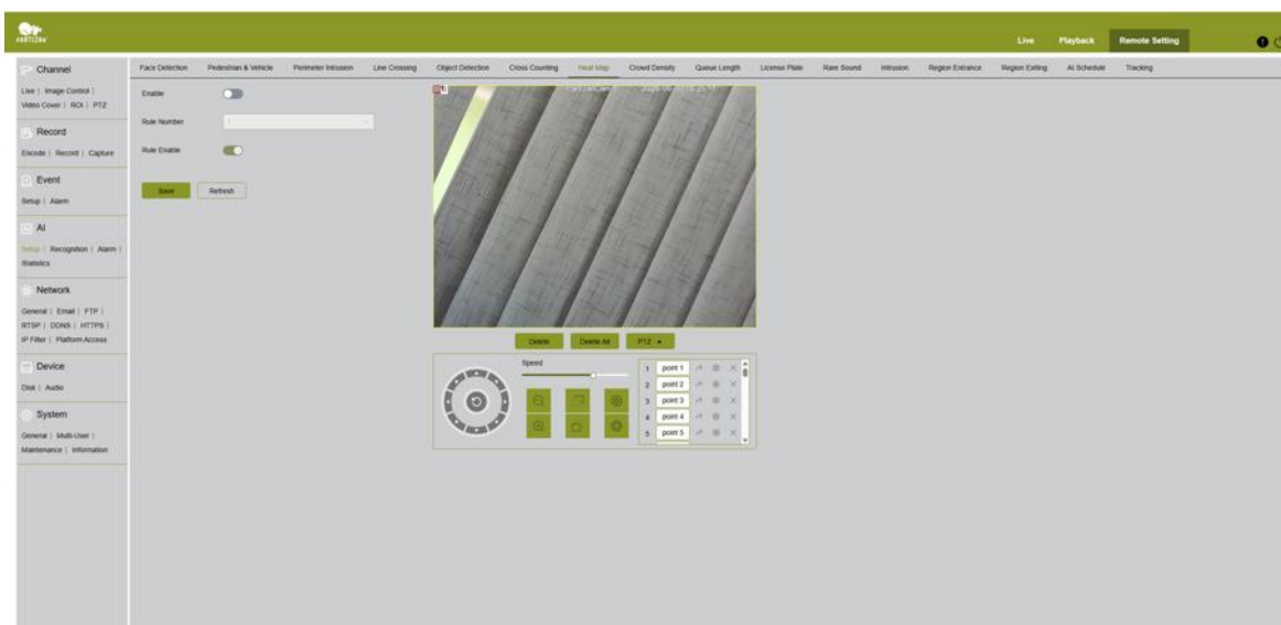
Fig. 44. AI → Setup → Heat Map — enables spatial activity density tracking for the selected rule region
