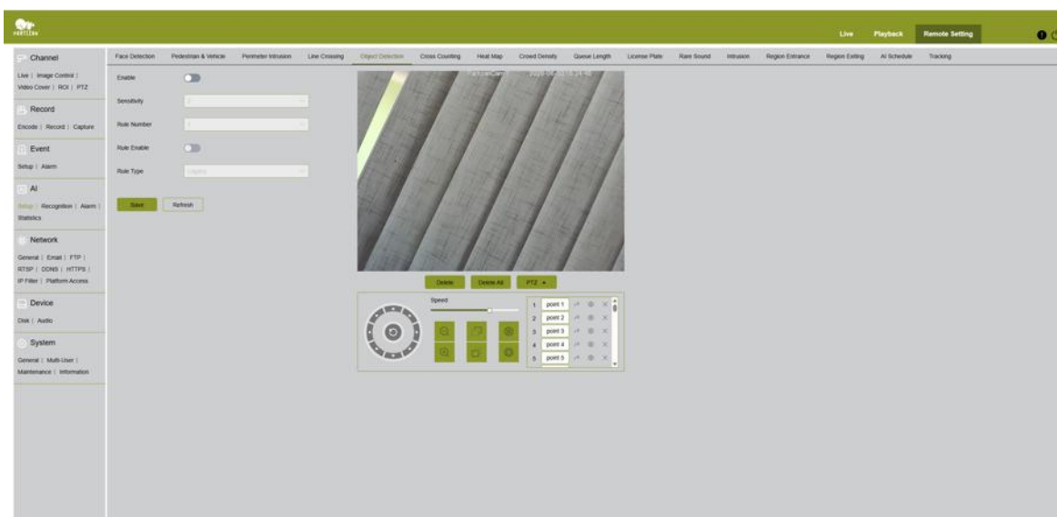
Fig. 42. AI → Setup → Object Detection — detects abandoned or removed objects within a defined rule area
